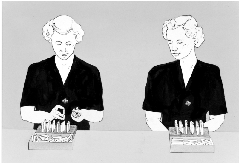
FIG. 6—The operator at right waits for her less productive self. Motion Studies Application (c. 1950)
