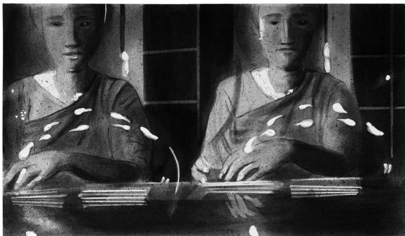
FIG. 4—Cyclograph study woman demonstrating light-tracking hand motions. First picture showing pointed spots, the spots showing direction. Frank B. Gilbreth (1914)
